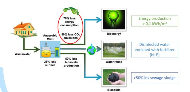
Figure 2: Anaerobic Treatment to Convert Wastewater to Methane - Graphic by Aqualia
